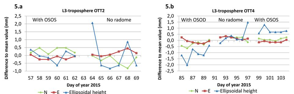
Figure 5: Time series with and without radome at the antennas. The coordinates have been computed with the same antenna model (calibrated model with OSOS for OTT2 and type model without radome for OTT4).
