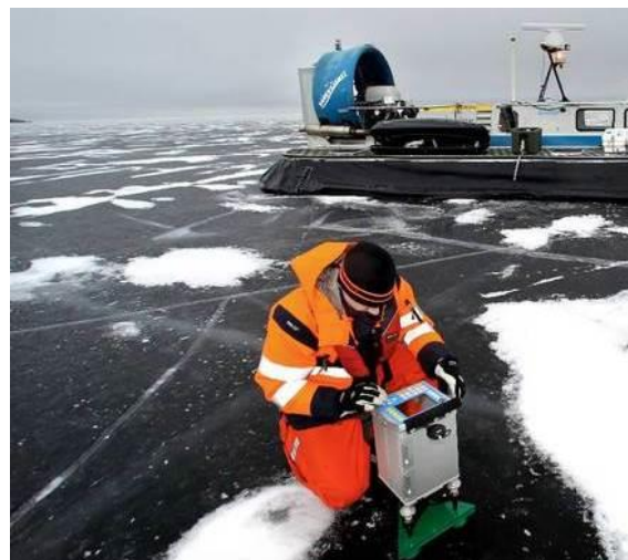
Figure 7.1: Relative gravity measurements in March 2011 on Lake Vänern, the largest lake in Sweden. Photo: Mikael Lindblom.
