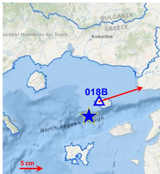
**Fig. 8** Estimated static horizontal displacement of station 018B. The epicentre of the earthquake is marked by blue star.
