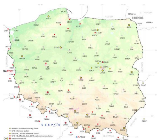
Fig. 18. Reference stations of the ASG-EUPOS system (14 April 2014)
