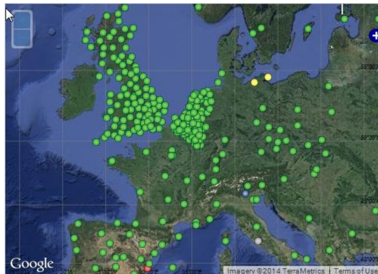
Figure 2: Real-Time GNSS network processed for severe weather monitoring (Status: 6 May 2014 some stations are located outside the region represented by the map).
