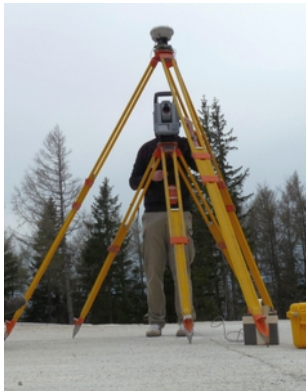
Simultaneous observation 24h-GPS and terrestrial
