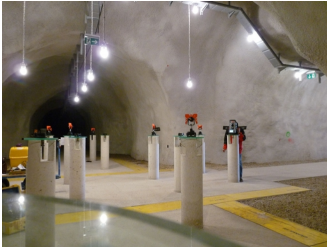
Pillars for geo-magnetic observations
