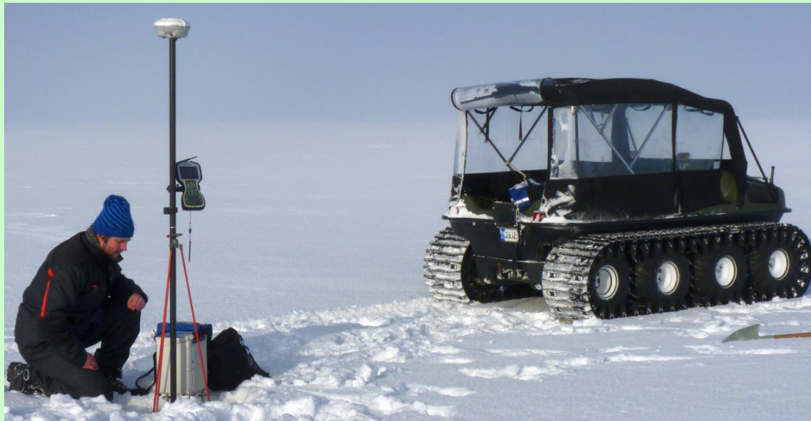
Fig. 4. Gravity survey in Väinameri in Winter 2013. Special lightweight crawler was used for transportation of 3-person team and equipment on ice with thickness of about 40 cm
