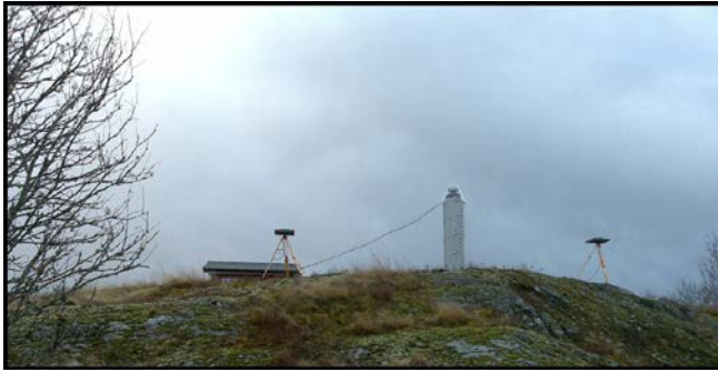
Figure 3. SWEPOS antenna at Vänersborg together with two reference antennas.
