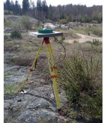
Hälsjöholm, 2010. One of the benchmark set-ups. An Eccosorb plate is mounted directly below the choke ring antenna. The GNSS receiver is kept in the SWEPOS equipment cabin during the campaign.
