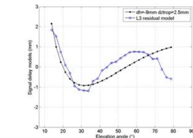
Fig 5. The black curve is constructed from three different curves giving the same bias effect on height difference, troposphere and clock bias, as the blue curve gives.
