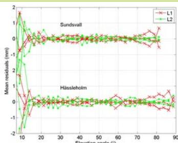
Fig 1. Phase residuals while computing between only the three reference antennas at two sites. The low noise (above 15° elevation) indicates good observations.
