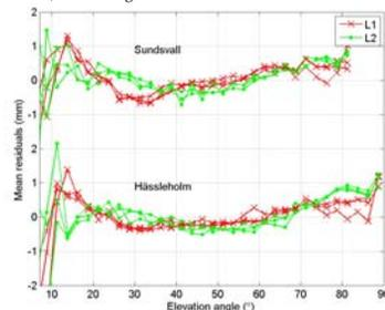
Fig 2. PCV values computed for the SWEPOS station individually from each of the three reference antennas at two sites. Good repeatability indicates that the method gives reliable results (at least above 15° elevation).
