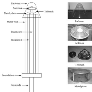
Principle design of a concrete pillar foundation in SWEPOS. Note the relatively large metal plate used as foundation for the tribraich. This may be a cause for disturbance. Designed 1992.
