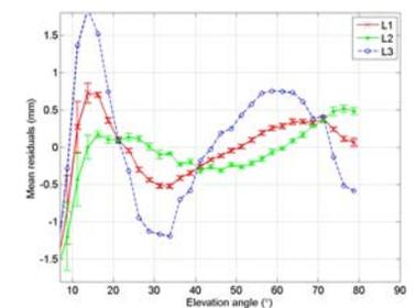
Fig 4. Mean of PCV in L1 and L2 for five sites, as well as computed L3 ionosphere-free linear combination (based on the values from L1 and L2). Note the amplification when forming L3.
