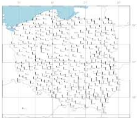
Fig. 8. Direct comparison of ETRF2000 (epoch 2011) and EUREF89 (epoch 1992) ellipsoidal heights
