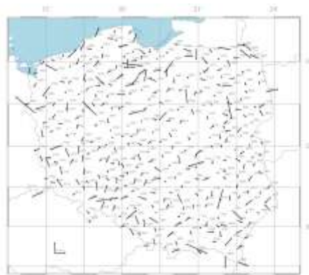
Fig. 9. Horizontal residuals obtained after 7-parameter Helmert's transformation between ETRF2000 (epoch 2011) and EUREF89 (epoch 1992)
