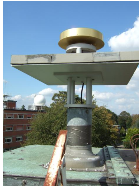
Fig. 1 – New BRUX station integrated in EPN/IGS as replacement of BRUS
