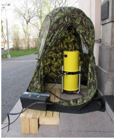
**Fig. 5.** The A10-020 at the station Turku Vartiovuori. Note the transportable benches and weights to mount the tent on stairs. Photo: Jaakko Mäkinen
