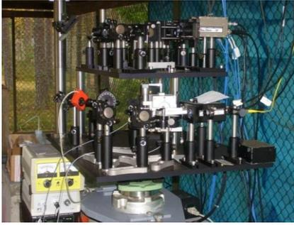
**Fig. 6.** A part of the new ADM equipment of the PTB on the zero pillar of the Nummela Standard Baseline. Photo: Jorma Jokela
