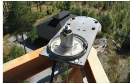
**Fig. 1.** The antenna on top of the 20 m high steel grid mast is stabilized with a special invar wire construction which eliminates the thermal expansion of the mast. Photo: Hannu Koivula
