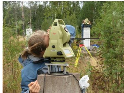
**Fig. 2.** Local tie measurements of METS GPS station with space intersection technique. Photo: Hannu Koivula
