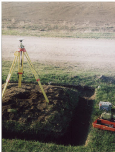
Combined Old Classical Triangulation and ETRS89 Control Points from GNSS measurements
