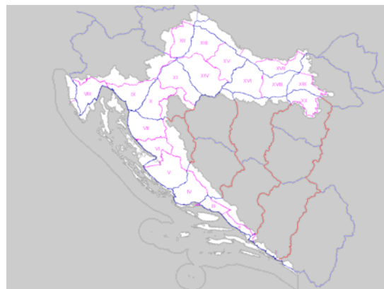
Fig 3 New levelling polygons (purple), old NVT lines (blue) and NVT lines across Bosnia and Herzegovina (red)
