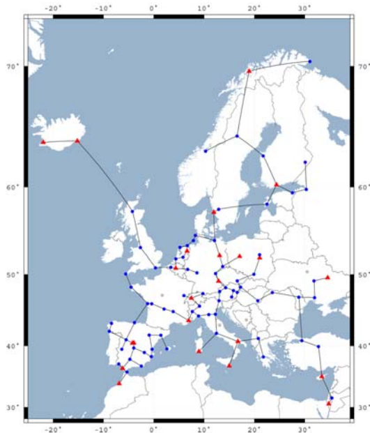
Figure 1. The analyzed network and the graph of the baselines generated in the batch adjustment: example of day 2009-263. Red triangles: reference IGS stations, blue circles: EPN stations.
