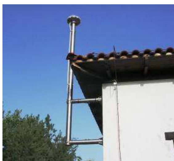
Figure 3: Typical installations of HEPOS stations: on roof (left) and on the side of the building (right).
