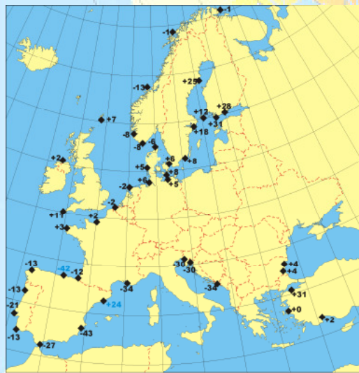
◆ Heights of the mean sea level 1997 above the GPS/Levelling quasi geoid of EUVN
