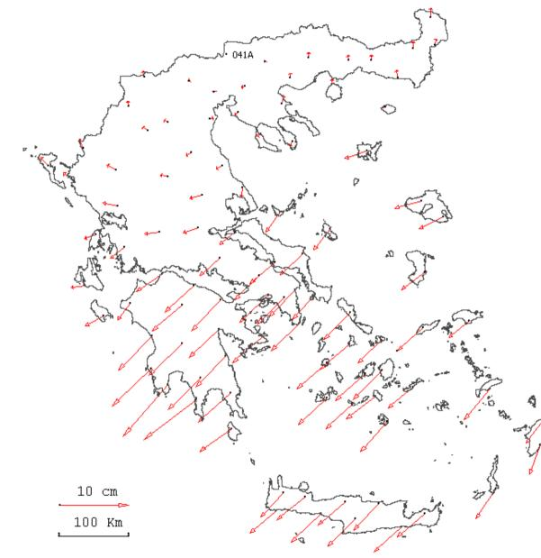
Displacements (in ITRF2005) of the HEPOS stations with respect to station 041A occurred from 11/2007 to 11/2009 (preliminary results)
