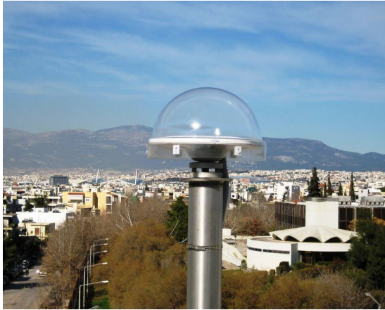
Fig. 3 A typical reference station of HEPOS.
