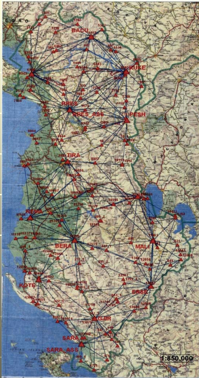
Fig. 3 GPS Static Network (RGN)
