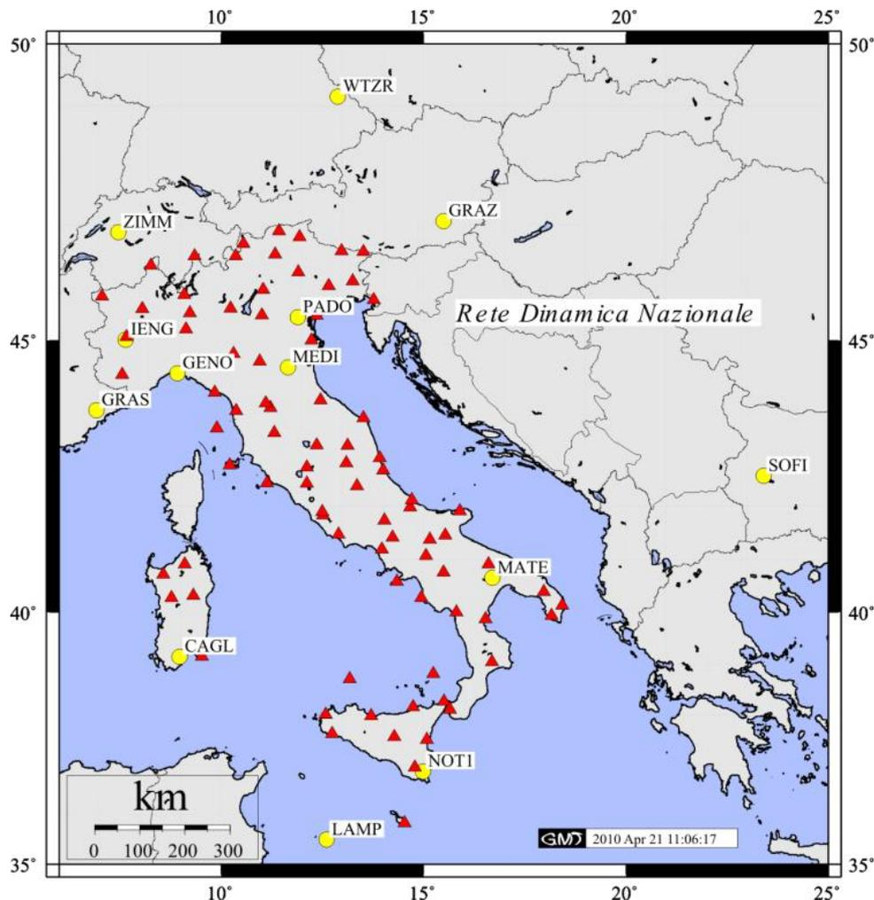
Figure 1 –The analyzed network: red triangles indicates the RDN stations and the yellow circles indicate the EPN EUREF stations used as reference stations
