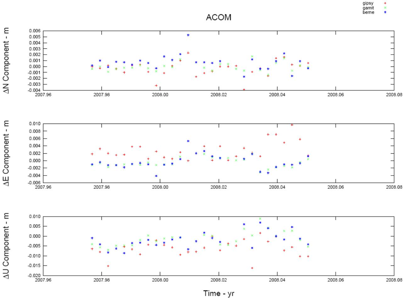
Figure 2 –Example of a time series obtained for the three software packages for one site (ACOM)
