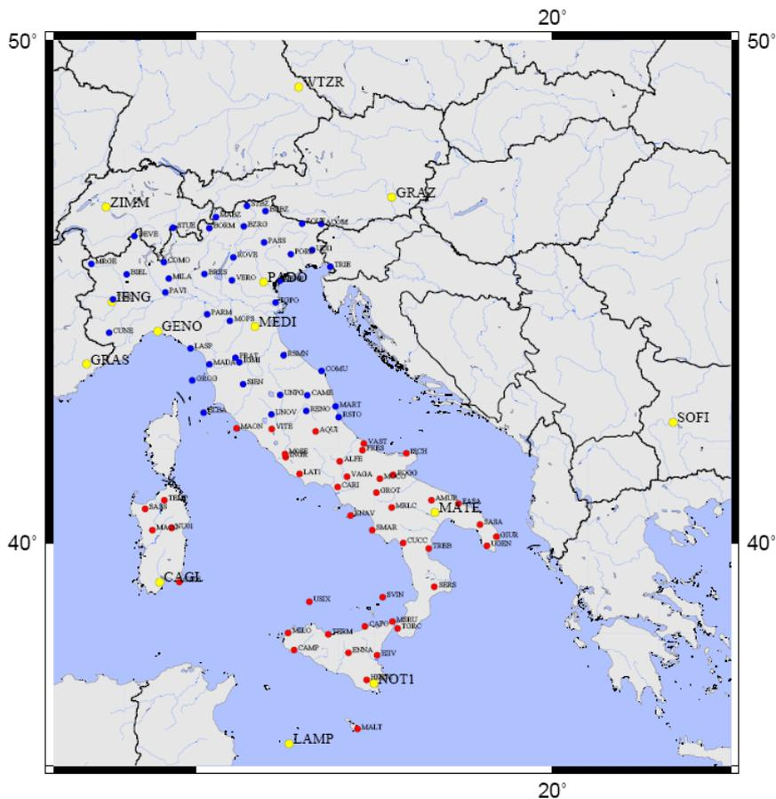
Figure 3 – Partitioning of the network into two clusters, north (blue dots) and south (red dots). Yellow dots represent common stations used in processing both clusters and in joining the partial solutions.
