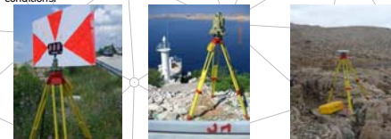
Figure 2: Devices for trigonometric and GPS levelling
