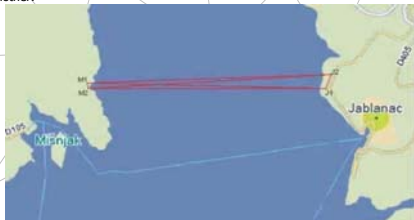
Figure 1: Network for height transmission between mainland and island Rab. It was necessary to attach the heights of the network stations at the bank side to the official levelling network. The additional application of a high precision levelling between network points at the same bank side in the combination with trigonometric levelling makes possible determination of the heights with higher accuracy and serves a reliable transmission of the heights over large water surfaces.
