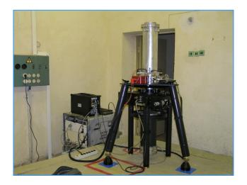
•The FG5 107 absolute gravimeter ran for 24 to 36 data sets, one set of 100 drops per hour
