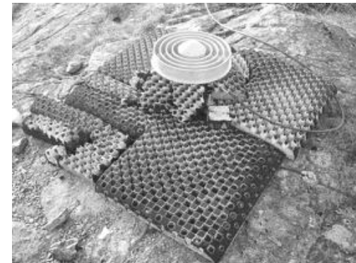
Reference antenna imbedded in ECCOSORB
