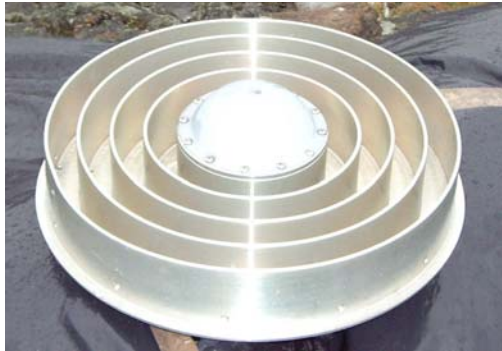
Dorne-Margolin antenna with choke ring ground plane
