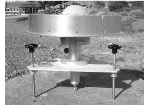
Reference antenna of type Dorn Margolin type T, together with used levelling device.
