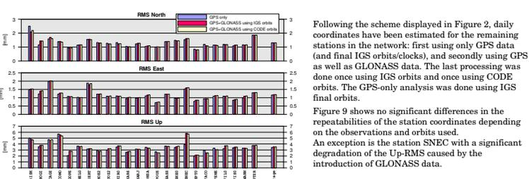
Figure 8: Coordinate repeatabilities obtained using GPS-only, GPS+GLONASS with IGS orbits, GPS+GLONASS with CODE orbits
