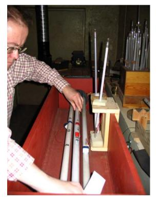
The quartz metre system with interferometrical comparisons in the Tuorla Observatory of University of Turku. (Photo: Pasi Häkli)
