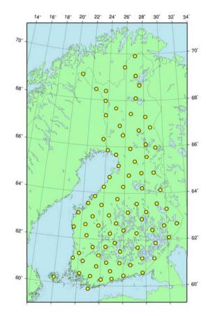
GPSNet.fi, Geotrim Ltd. 84 stations (11.6.2006) Recording interval 1 sec RTK, VRS and DGPS solutions
