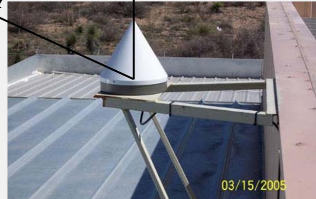
GNSS antenna at AZCO (with CONE radome)
