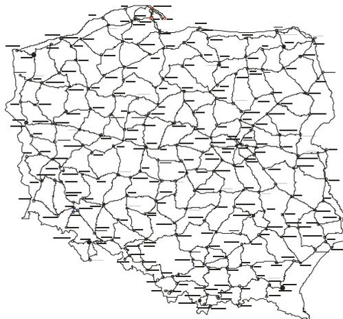
Fig. 2-1 Fourth precise levelling network in Poland (1999-2003)
