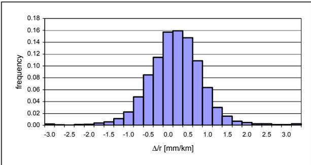
Fig. 2-2 Histogram of discrepancies  $\Delta/r$  for the complete levelling network
