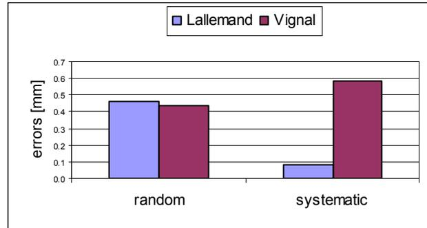
Fig. 2-6 Comparison of random and systematic errors computed from Lallemand's and Vignal's formulas for the first campaign
