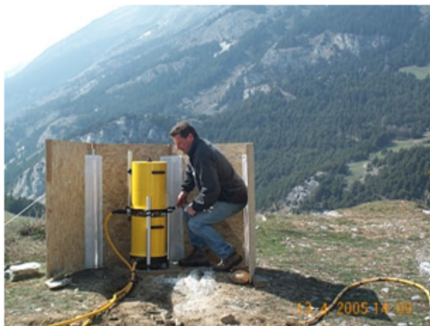
A10 gravimeter operated in the French Alps
