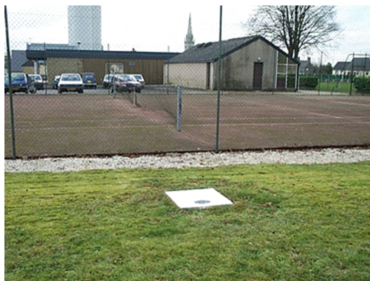
A standard RBF point, suitable for GPS and gravity measurements: 1 m 3 slab. The benchmark is protected by law and periodically visited.
