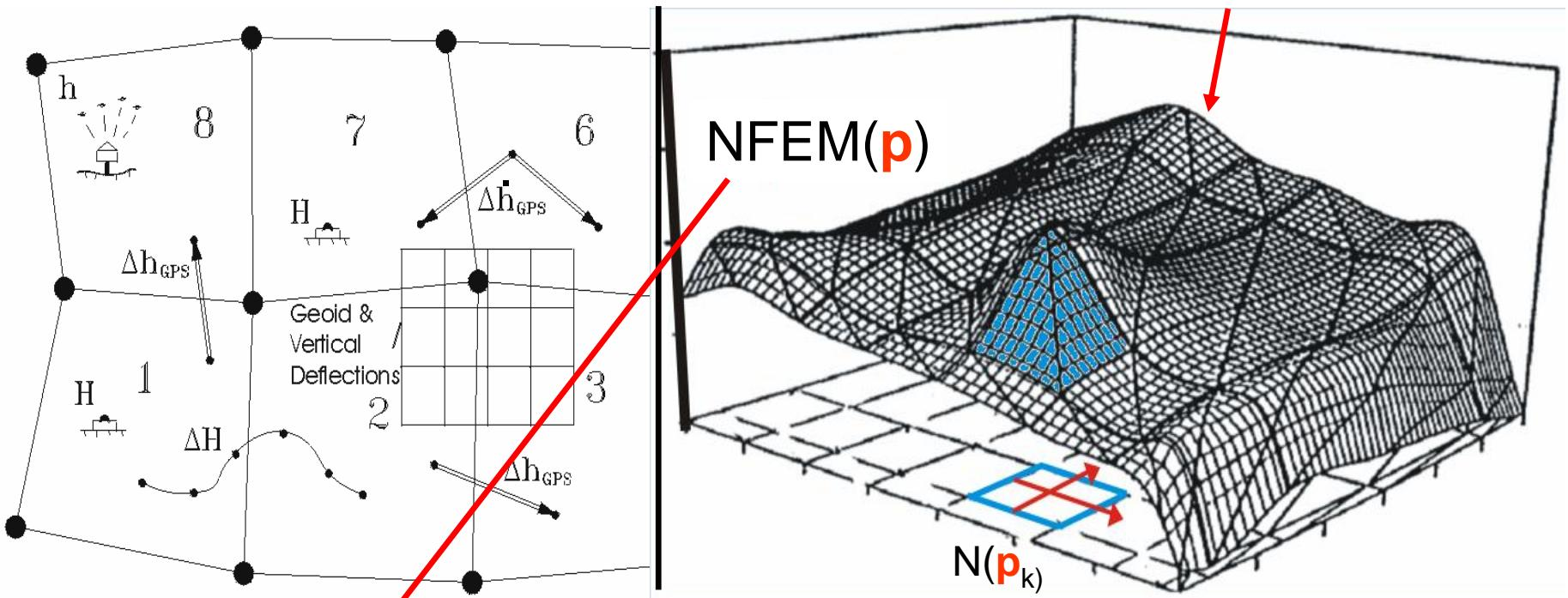
$$NFEM(\mathbf{p} | \mathbf{B}, \mathbf{L}) =: \left\{ \begin{array}{l} N(\mathbf{p}_k) = [1 \mid x \ y \mid x^2 \ xy \ y^2 \mid x^3 \ x^2y \ xy^2 \dots] \\ [p_{00} \mid p_{10} \ p_{01} \mid p_{20} \ p_{11} \ p_{02} \mid p_{30} \dots]_k \\ = \mathbf{f}^T \cdot \mathbf{p}_k \\ + \text{ContinuityConditions along the Borders} \end{array} \right\}$$
