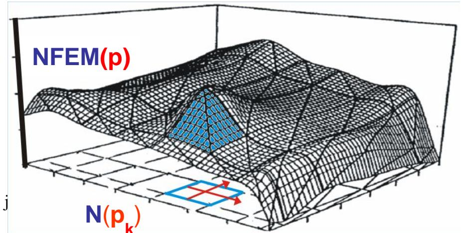
$$\frac{a}{4\pi\gamma(B)} \iint_{\sigma} Dg \cdot S(\psi) d\sigma + v = \mathbf{NFEM}(p) = f^T \cdot p$$
