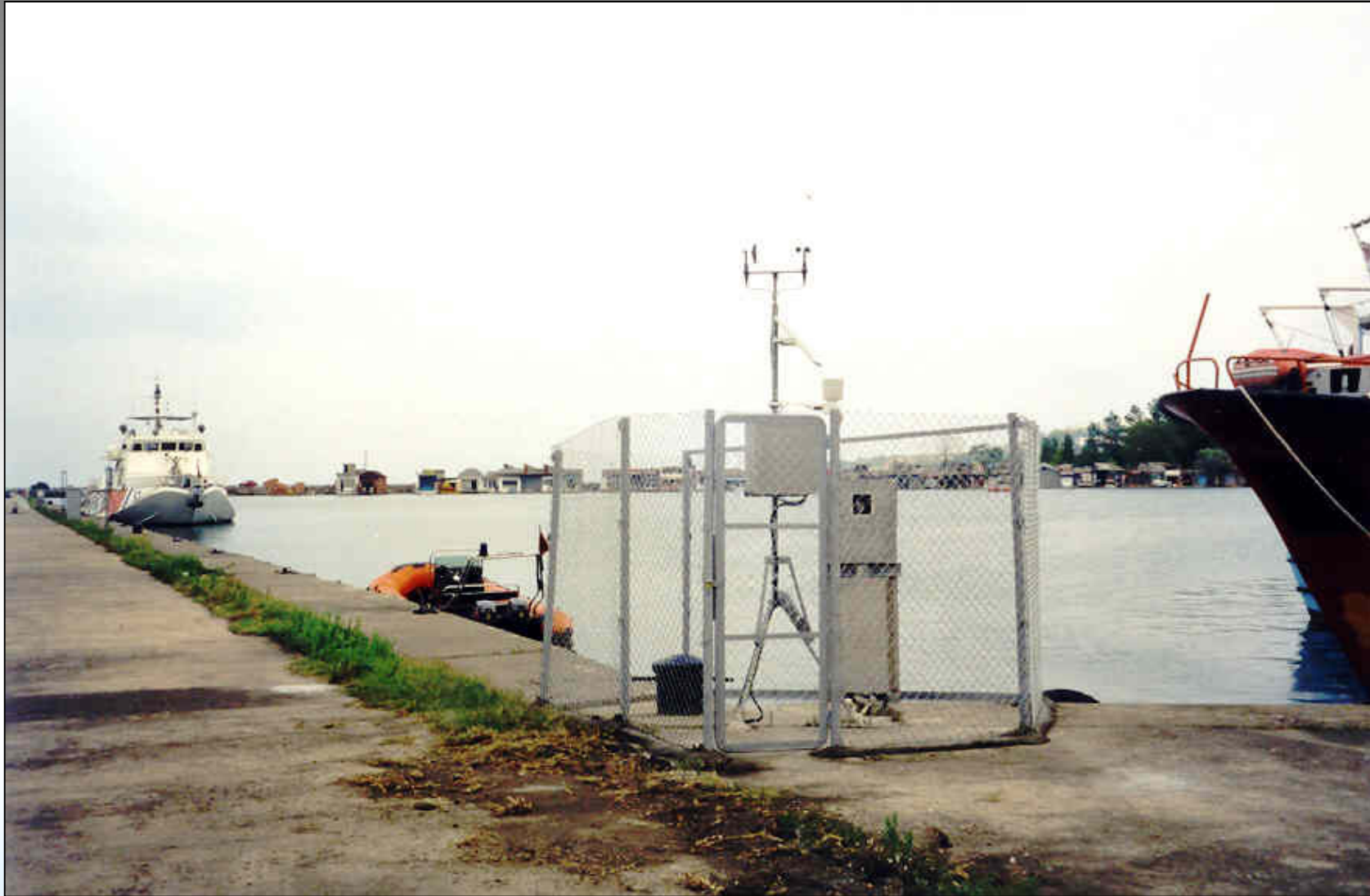
➤ Trabzon-II digital and automatic tide gauge
