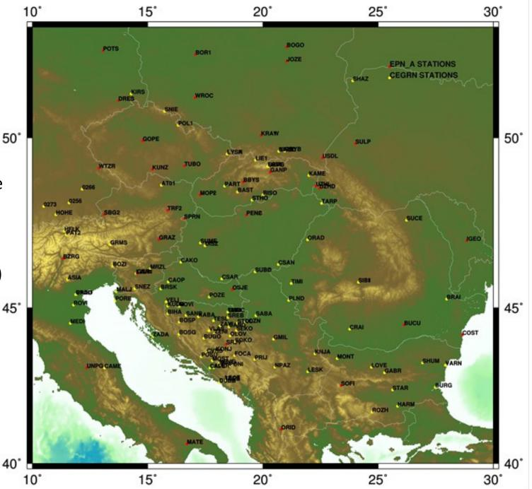
CEGRN sites in the context of the EPN\_A sites used for alignment to ETRF2000 (C1725)
