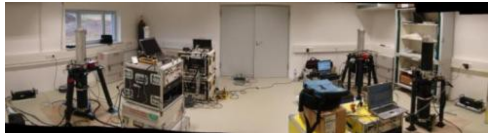
Comparison experiment with five absolute gravimeters
