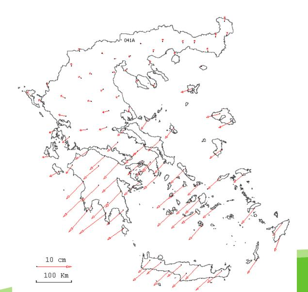
Differential displacements of the HEPOS stations over two years(w.r.t. station 041A, 11/2007 -11/2009) (Gianniou, 2010)
