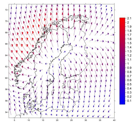
Horizontal (0 to 2 mm/yr): The GIA model in Milne 2001 transformed to the GPSvelocities (in Lidberg 2007). Vertical (-1 to 10 mm/yr): The NKG2005LU(ABS) model Based on: TG, repeated levelling, and GPS. (Ågren & Svensson 2006)
